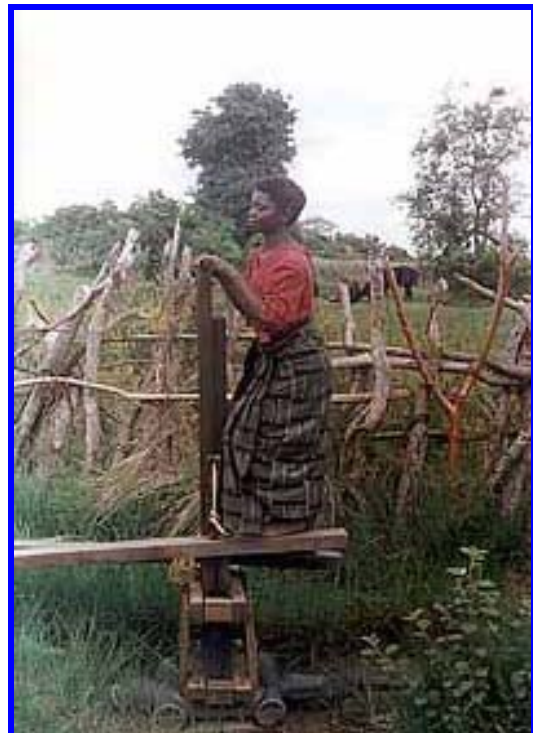
TREADLE PUMP IN ZAMBIA - A SOLUTION FOR THE URBAN SECTOR AS WELL (Source FAO
